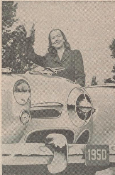
FRONT END DESIGN OF THE NEW 1950 STUDEBAKER MODELS IS PARTICULARLY STRIKING. THE "SPINNER," IN ADDITION TO PROVIDING A HANDSOME ORNAMENTAL TOUCH, AUGMENTS FOUR FRONTAL OPENINGS WHICH DIRECT AIR TO THE ENGINE. THE LARGEST OF THESE AIR PASSAGES CONSISTS OF TWO OVAL-SHAPED HONEYCOMB GRILLE SCOOPS LOCATED BELOW TWO SMALLER AIR CHANNELS WHICH FLANK THE "SPINNER."
